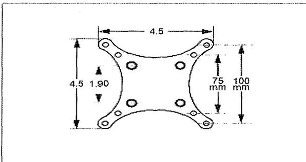
This so-called "Star" VESA plate is our most commonly used VESA adaptor. It accommodates most small to mid-size monitors with 75 x 75 mm and 100 x 100 mm VESA hole patterns. The adaptor fits to a tilter mechanism utilizing the 1.9 x 1.9 inch inside holes. The device measures 4.5 x 4.5 inches in size. For monitors with recessed VESA hole patterns an additional VESA Spacer hardware kit may be needed.
